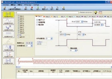
"Quick Immunity Sequencer 2" (model name: SD009-PCR-LE) is an application software for immunity testing with the AC power supply PCR-LE series system, based on the power line disturbance standard (IEC61000-4 Series) for the immunity testing of the EMC standard.
