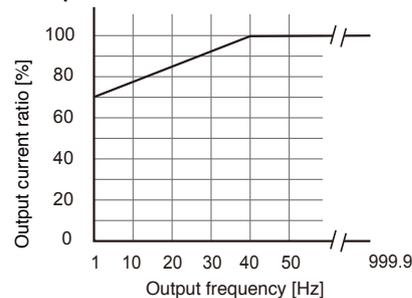
For the "Output voltage ratio versus rated output current characteristics (AC mode)" and "Load power factor versus rated output current characteristics" graphs, the rated output current is the product of output current ratios shown in both graphs. The output current ratio shown in the "Output frequency versus rated output current characteristics" graph is given priority if it is less than the product of output current ratios described above. (This only applies to AC mode.)
